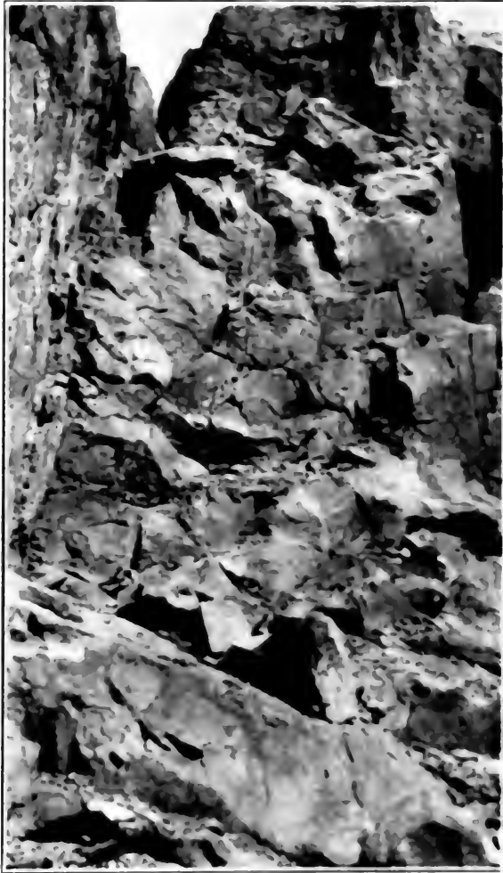
Open cut in Huronian conglomerate, Coniagas Mine, Cobalt — At extreme left are two narrow vertical silver-smaltite veins
